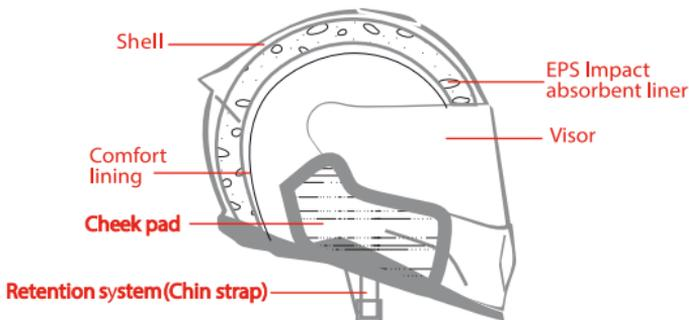
The main function of the helmet is to protect your head in case of impact. This is accomplished by the shock absorbing capacities of various types of materials and different densities of the EPS.
